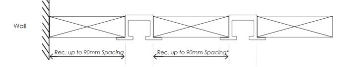
5. **Double Track:** The spacing from the wall and between the tracks can be up to 90mm.
