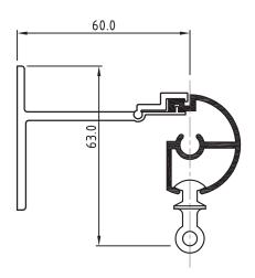
Base Plate : Height 50mm, Width 30mm Top of base plate to hook (or ⊄ snap) position : 63mm
