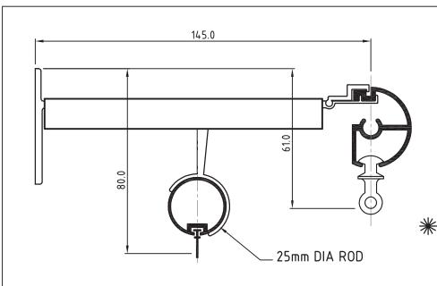
Base Plate : Height 50mm, Width 30mm Top of base plate to rear hook position : 80mm
