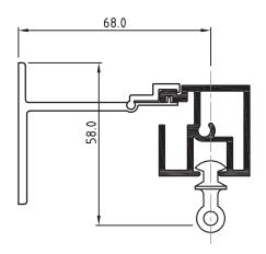
Base Plate : Height 50mm, Width 30mm Top of base plate to hook (or ⊄ snap) position : 58mm
